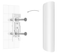
• **To mount a small magnet:** remove the front panel using a plectrum or plastic card. Fix the part with magnets on the surface; use the bundled screws for this. Then install the front panel on its place.
