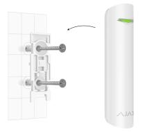
• **To mount a large magnet:** remove it from the SmartBracket mounting panel. Then fix the SmartBracket panel with bundled screws. Install the magnet on the panel.
