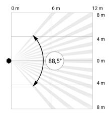
If the detector is not installed at the recommended height, this will reduce the area of the motion detection zone and impair the operation of the function of ignoring animals.
