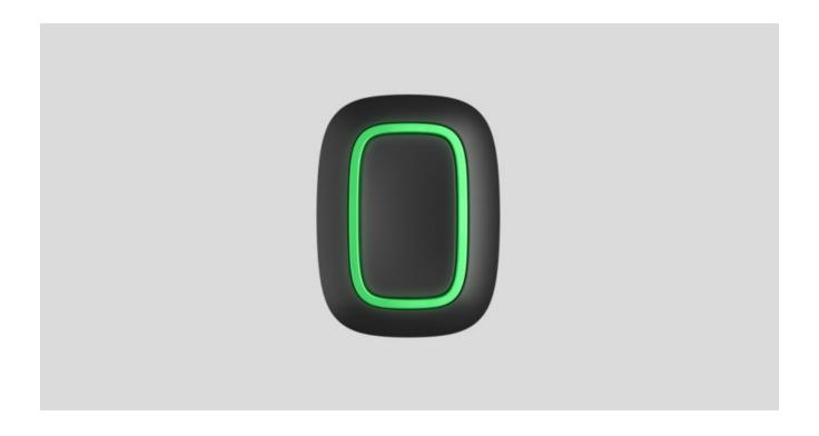
**Button** is a wireless panic button with protection against accidental press and additional mode to control automation devices.
