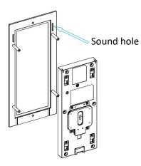
Combine the device with the flush-mounting bracket according to the direction indicated in the figure.
