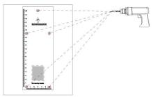
Stick the wall-mounting template onto the wall according to your need. Then use an electric drill with a 6mm diameter bit to make five holes with 20mm depth according to the hole of wall-mounting template.
