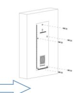
Insert five plastic wall anchors into the holes.
