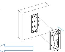
Combine the flush-mounting bracket and flush-mounting rain cover. Then align the fixing holes of flush-mounting bracket with the fixing holes of flush-mounting box, and use torx wrench to tighten flush-mounting plate with two M4x16 torx head screws.
