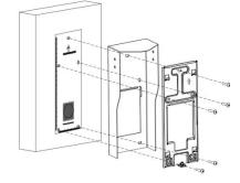
Put the wall-mounting bracket into the rain cover, and please align the bracket's screw holes with the screw holes of rain cover. Then tighten the combined wall-mounting bracket and rain cover on the wall with five ST4x20 crosshead screws.
