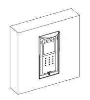
Check if the gap surrounding the device is even and securely installed. Make sure to reserve a gap and power on the device to check the device is normal. Installation is completed.
