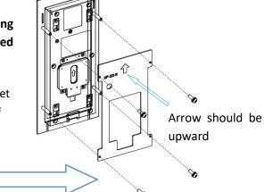
Align the fixing hole of flush-mounting plate with the bolts of flush-mounting bracket, then insert flush-mounting plate onto the flush-mounting bracket. Use four M3x8 crosshead screws to fix flush-mounting plate.
