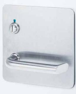
The 202 Series Door Furniture is 162mm square with 10mm radius corners. Concealed fixed plates have studs with internal threads located in each corner, visible fixed plates have corresponding countersunk holes and are fixed back to back through the door.
