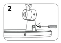
Take the screw from the base and tighten them with a screwdriver.
