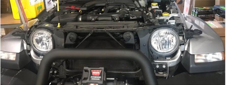
2. Next, remove the 3 bolts holding stock headlight brackets in place to remove the headlight assembly using a 10mm socket. Unplug the headlight from the OEM harness and remove assembly. Repeat for other side.
