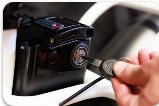
Key angled = OFF position Key vertical = ON position
