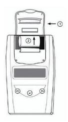
How to replace the paper jam Step 1: open the clear cover Step 2: pull the paper slowly and straightly from the paper roll in the chamber
