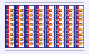
**Below 380°F** - safe and normal running temperature, not registering on label **380-435°F** - running hot but still OK, inspect and change seals more frequently **450°F and above** – running very hot, replace seals and inspect immediately
