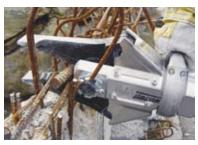
The HCS 6 **C** is specially designed to expand and separate material, e.g. ripping radiators or door frames from walls or breaking up concrete pieces. The tool has a shear set for cutting-up various materials, like reinforcements up to 20 mm (0,8 inches) in diameter.
