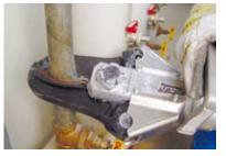
The HCS 6 **S**, equipped with sickle shaped blades, is able to cut sheet metal, piping, high voltage cables, rebar (up to 16 mm/ 0,6 inches in diameter) and wooden frames. The sickle insures that the material can't slip out.
