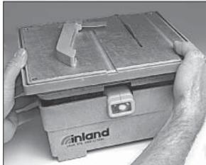
to make sure there is no interference between the blade, guard, and the work surface by plugging in the saw and turning the switch on and off quickly. The saw should run smoothly and quietly. If the blade makes contact with anything repeat Steps 4-6 until it turns properly.
