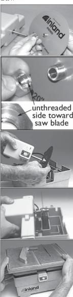
to make sure there is no interference between the blade, guard, and the work surface by plugging in the saw and turning the switch on and off quickly. The saw should run smoothly and quietly. If the blade makes contact with anything repeat Steps 4-6 until it turns properly.
