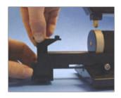
3. Next, press the turntable support (B) into the square opening at the front end of the rail assembly. For small circles, it should be inserted with the turntable bearing pin (C) toward the drive wheel. The distance between the cutter wheel and center of the bearing pin is the circles radius. If your unit is set up on a surface grid, leave the rubber foot (K) off the bottom of the support post.
