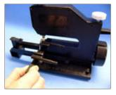
1. First, position the main rail assembly so it extends out about half way. Place the straight edge guide (G) into the throat of the cutter.
