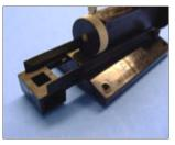
1. Place the main rail assembly (A) on the cutter. There is a small guide rail on each side of the cutter body near the base of the unit. The track assembly slides onto these rails with the square block down. Note that if you purchased the ScoreOne<sup>TM</sup> Plus, the rail and turntable are already installed and you can proceed to the "Scoring Circles" section below.
