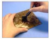
5. Depress the lever again and lift the glass and turntable off the support pin and remove it from under the cutter. The plastic pry bar (J) is then inserted in the bearing hole at the bottom of the turntable and pressed sideways to remove it from the glass. Be careful to use slow, steady pressure to prevent cracking the glass. Your ScoreOne<sup>TM</sup> Glass Cutter has completed its work. Now you must break out the circle from the surrounding glass.
