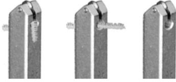
**Cutting Head:** The cutter head has a hole that inserts into. This hole removes accumulated glass chips and cutting debris and lubricates the cutting wheel axle. Keeping the wheel free turning is important to producing a good score.
