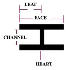
Metal cames are available in zinc, brass, and copper. "H"-shaped is used between two pieces of glass. "U"-shaped and "Y"-shaped came is most often used on the perimeter of a piece. Both "U" and "Y" are available in adjustable versions when working with different thicknesses and uneven edges.
