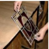
With a sweeping motion, bring the panel from the horizontal position to vertical while keeping the middle of the panel supported by the edge of the table.
