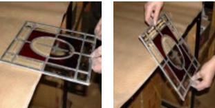
Slide the panel toward you until it rests half on and half off the table. The edge of the table should run through the middle of the panel.
