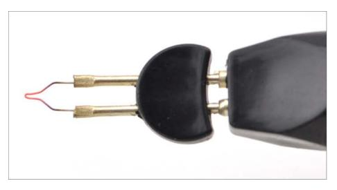
Press down on the ON/OFF Switch to check the battery has been installed correctly and that your heating element gets hot. ALWAYS let it cool down before touching it. And always remember the element is extremely fragile and can be damaged or broken by just the slightest jiggling. Now we are ready to singe! Let's try it on a macramé project, like <u>Easy Wrap</u>.
