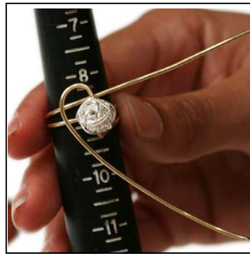
Step 11 To ensure the right size, slip the ring onto the ring mandrel and push it down to the right size.
