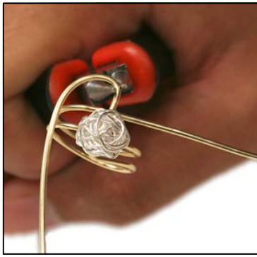
Step 10 Use the wire to start creating the nest. Use either round-nose pliers, or your hands.
