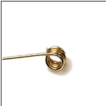
Step 5 Continue to coil until you have 3-4 coils. Make sure your coils are tight and consistent.
