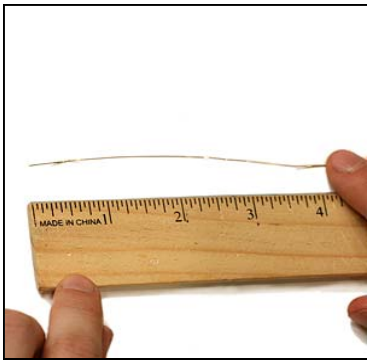
Step 1 Cut wire into 4 inch pieces.
