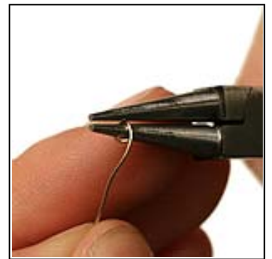
Step 4 Begin to coil starting at the tip of the wire using the middle of your round nose pliers. Be sure to make the coil big enough to thread onto the leather.
