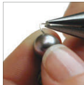
Step 9 To open or close a rosary loop, lift the loop out of its plane. Do not pull the loop open sideways or you will distort its round shape.
