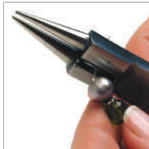
Step 3 Using the cutter portion of the rosary pliers, remove excess wire leaving about 3/8".
