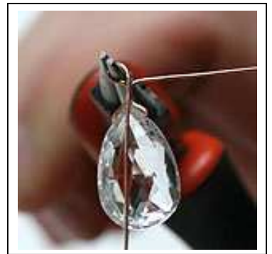
Step 8 Rotate your round nose tool and continue to bring your wire into a loop.
