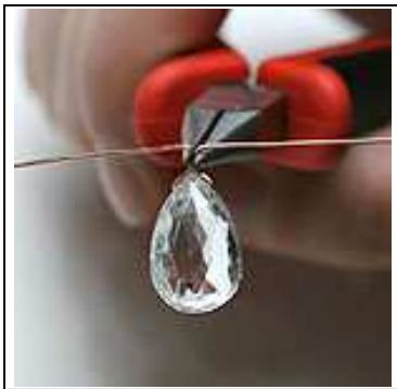
Step 5 Bend the two wires to a right angle in opposite directions.
