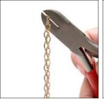
Step 1 Begin by folding the 26" - 28" length of chain in half and cutting it into two even segments.
