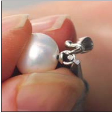
Step 24 Use the tip of your round nose pliers to carefully curve the wire down into the bowl of the end tip. Make sure the hook securely rest inside the bowl. Repeat on the other side.
