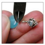
**Step 17**Use the wire cutters to clip off excess wire.
