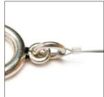
**Step 7** The finished result should be a rounded compact crimp.
