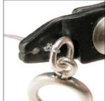
**Step 5**The result should be a slightly rounded crimp with a dip running down the center.
