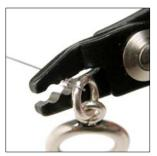
**Step 4**Enter the crimp bead in the first channel of the crimping pliers and crimp firmly.
