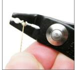
Step 3 Place the crimp bead into the inner jaw (lipshaped hole) of the crimping pliers.
