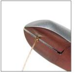
Step 7 Use the wire cutters to trim off the short stringing wire so it is flush with the crimp bead.
