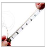
**Step 29**Measure 7" up the wire on both sides from the "V".
