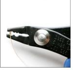
Step 5 To fold the hammock in half, place it into the outer jaw (oval-shaped hole) of the crimping pliers.
