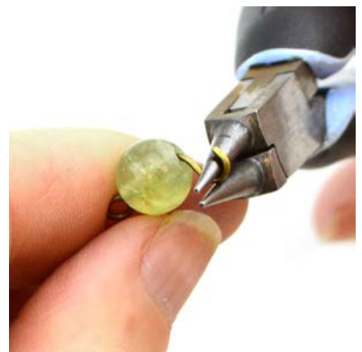
Step 6. Loop the wire up and over, (towards the bead) keeping the wire as straight as you can over the center of the bead. Shape the loop in a series of quarter turns, feeding the wire through the heads of the pliers.
