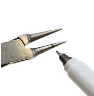
Step 4. Use a fine tip permanent marker and mark head of the round nose pliers. This will allow you to size your loops consistently throughout the project. For a 3/8" wire tail, mark about 1/4" from the tip of the pliers.
