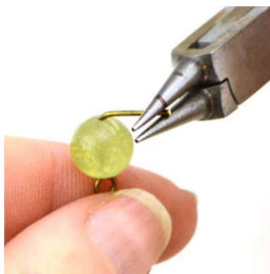
Step 5. Grip the very end of the wire with the round nose pliers. The end of the wire should be in line with the mark on the pliers.
