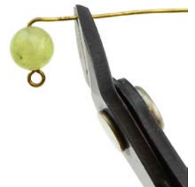
Step 3. Cut away excess wire with flush cutters leaving a 3/8" tail.
