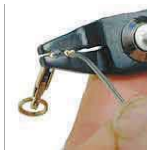
Step 4 Enter the crimp bead in the first channel of the crimping plier and crimp firmly.
