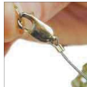
Step 5 The result should be a slightly rounded crimp with a dip running down the center.
