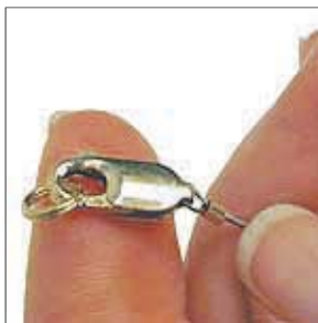
Step 3 Slide crimp bead up towards the clasp leaving a small loop that is large enough to allow movement of the clasp.
