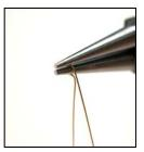
**Step 5** Take the loop out of the top plier nose and place it around the bottom plier nose.
