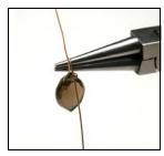
**Step 24** Bring the bent wire up and over the top nose of the plier.
