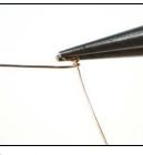
**Step 8** Wrap your wire 3 times around the longer wire, starting from the bottom of the loop. Trim the excess wire from the wrap.
