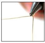
**Step 6** Bring the same wire underneath the bottom nose of the plier. You have now created a complete loop.
