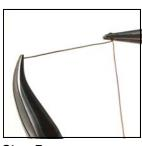
**Step 7** Hold the loop with your round-nose pliers and the short wire with your bentnose pliers.
