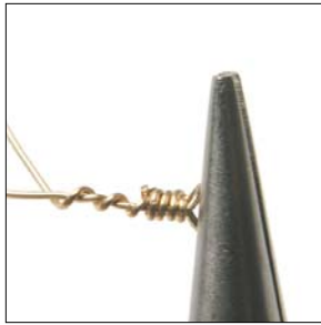
Step 17 Twist the wires so they become interwine. Repeat until you get about 1/2-1" of twisted wire.
