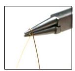
**Step 30**Bend the wire over the top of the pliers
