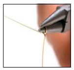
**Step 32**Pull the wire underneath the bottom plier and away from you, finishing the loop.
