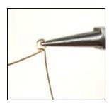
**Step 33** With your round-nose pliers, gently grab onto the loop so it is slightly opened.
