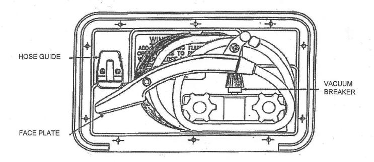
Please use care when using the shower hose. It is connected to the faucet through a code approved vacuum breaker. Breakage of the vacuum breaker through customer abuse is not covered under warranty. Replacement vacuum breakers are available. Part #25L53VAC.
