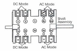
B. The RM2510/RM2610/RM2810 selector switch should be checked for continuity in the following manner. Remove all wires from the assembly. For the DC mode, continuity should exist between terminals 1 and 1A and 2 and 2A. For the gas mode, you should have continuity between 3 and 3A.
