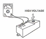
Next, disconnect DC power at the terminal block. Remove high voltage cable from igniter. Reconnect DC power, the igniter should produce a sparking sound. If not, replace the igniter.
