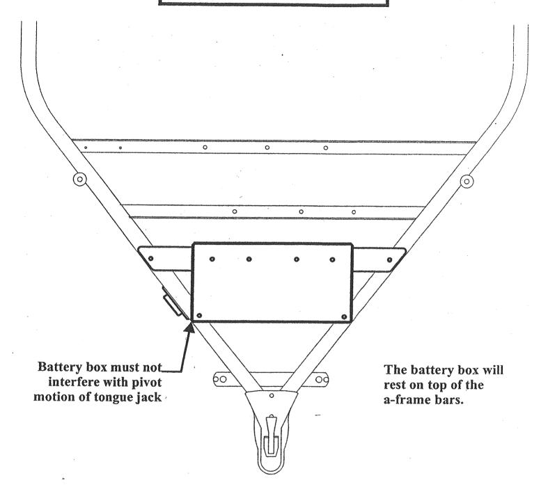
This battery mount kit can only be used on trailers equipped with the black (Norco) tongue jacks. The silver (Atwood) tongue jacks are not tall enough to clear the battery when installed.
