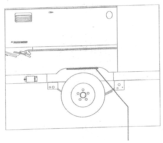
16" VELSTICK (APPLY TO BODY PANEL FLANGE FACING DOWNWARD) INSTALL WITH THREE SCREWS PROVIDED. VELSTICK SHOULD BE FLUSH WITH OUTER EDGE OF WHEEL WELL.
