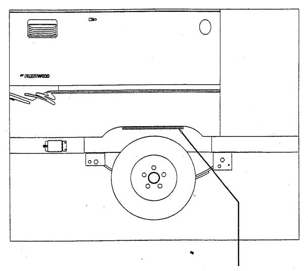
16" VELSTICK (APPLY TO BODY PANEL FLANGE FACING DOWNWARD) INSTALL WITH THREE SCREWS (4737-848). VELSTICK SHOULD BE FLUSH WITH OUTER EDGE OF WHEEL WELL.
