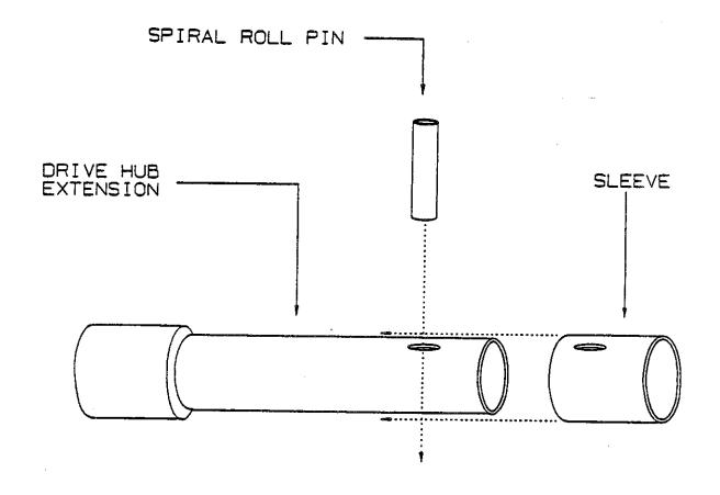
STEP 1: SLIDE SLEEVE OVER DRIVE HUB EXTENSION, ALIGNING HOLES ON DRIVE HUB EXTENSION WITH HOLES ON SLEEVE.
