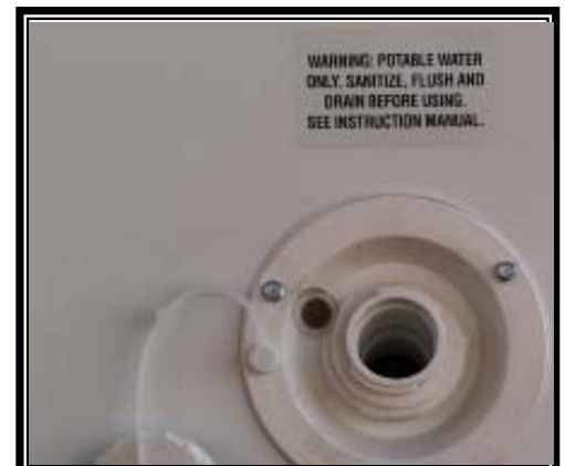
Exterior Water Fill Spout
