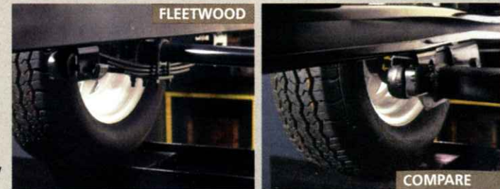
The above photos are for illustration purposes only. They depict demonstrations conducted by an independent testing and research laboratory and illustrate a result of applying a 10,000lb force to a tubular frame member mounted leaf spring and axle used by Fleetwood, and a C channel frame member mounted torsion axle similar to many competitors.
