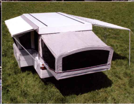
Exclusive AlumiTite™ Composite Roof features an awning rail on both sides of the trailer for optional canopy and sun shade. (Sun shade not available on Destiny Series)
