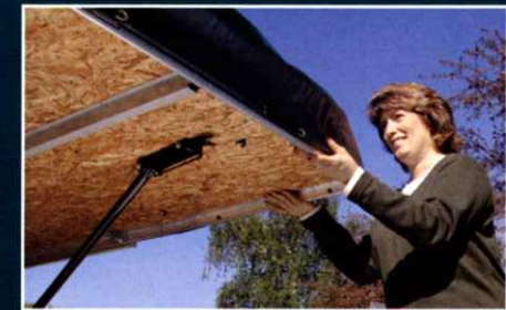
BackSaver™ bed support system makes set-up easier. Simply engage the support leg onto the bumper and lift the bed slightly until the support locks into place...that's it, you're done!
