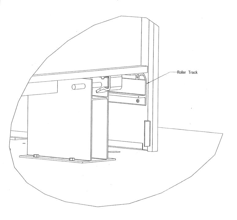
DETAIL OF GLIDE-OUT SHOWING CLIP DISENGAGED FROM ROLLER
