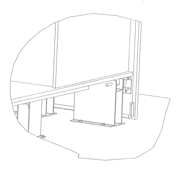
DETAIL OF GLIDE-OUT SHOWING CLIP ENGAGED ONTO ROLLER
