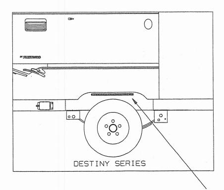
16" VELSTICK Install with two screws (4737-848) Flush with outer edge of wheel well
