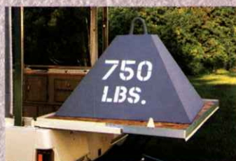
Each end bunk is engineered to support 750 lbs.
