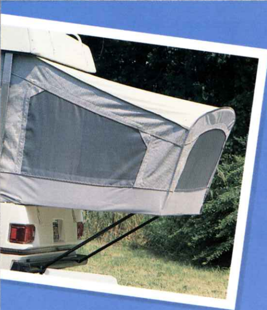
Conestoga-designed end bunks are angled to permit air flow and cross ventilation inside your trailer even in a heavy rain storm.
