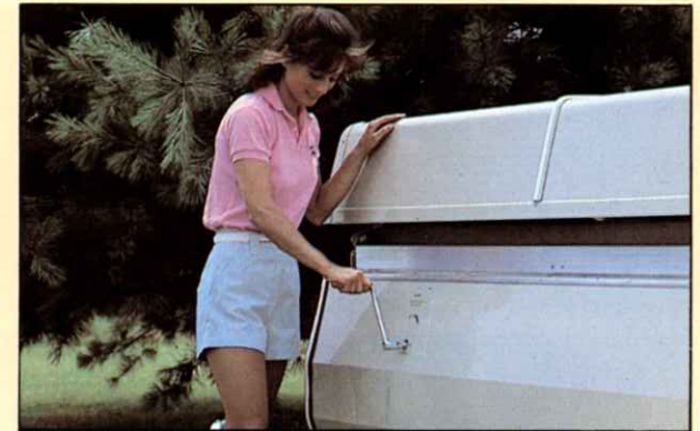
Coleman's exclusive waste-level crank gives you better leverage for raising the trailer and eliminates awkward stooping and kneeling.
