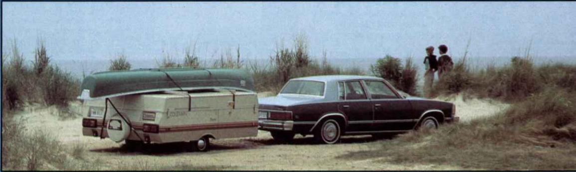
Boat/luggage rack enables trailer to carry a boat, canoe or extra luggage; distributes weight evenly over the trailer.
