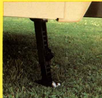
❑ 4. Self-storing Posilok stabilizer —securely levels camper on uneven terrain; standard on all models.
