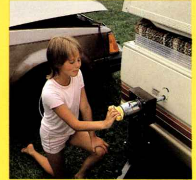
4. Electric lift —battery-operated motor electrically raises and lowers the roof.
