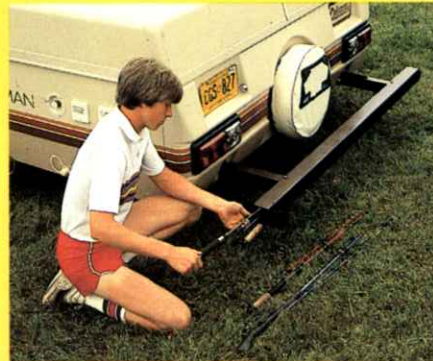
6. Heavy-duty storage bumper —for added trailer protection, choose a split bumper or the one-piece storage bumper.
