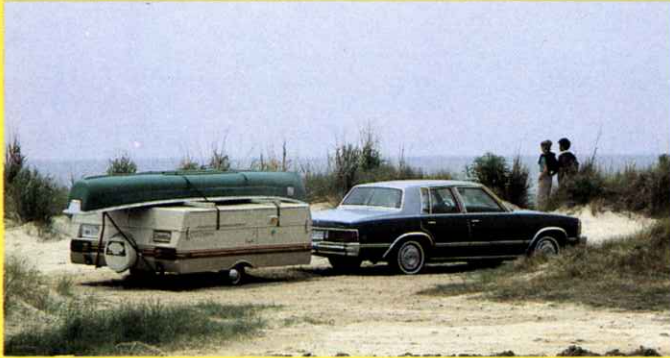
1. Boat/luggage rack —enables trailer to carry a boat, canoe or extra luggage; distributes weight evenly over the trailer.
