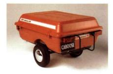
The body is molded in one piece from tough high-density polyethylene, the same material we use to make the world's largest-selling canoes. So is the optional all-weather top. That means the Caboose won't rust or rattle.
