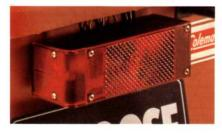
High-mounted tail/brake lights are clearly visible, yet protected by the "bumpers" from accidental bumps when you're backing up. The bumpers also serve as a base when you stand the Caboose on end for storage.
