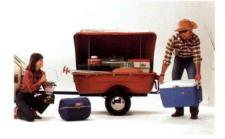
The top is hinged to open from either side, with two supports to keep it open securely. Closed, the supports fit into a body bracket to keep them handy and rattle free.
