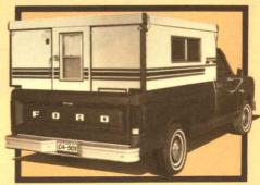
Low profile for roading. Fold up the sides, lower the roof, and you're ready to go with minimal wind resistance. You can also pull a boat and trailer without breaking "double trailering" laws.
