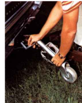
Flip-up dolly jack features attached wheel that swings up to avoid low-spot towing scrapes.
