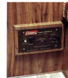
A 12V converter, standard on all models but the Rebel, lets you choose battery operation or 115V electrical power for lights and appliances.
